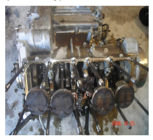
Now, remove the starter from the motor. 2 bolts hold it in, then you just kind of wiggle it out. inside the peanut cover (where the starter/idle gear is) you will see a small gear with a rod in the center. Remove this gear and rod, place it somewhere safe.
